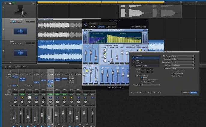
If your chosen reverb plug-in doesn't feature its own EQ controls, you can insert an EQ plug-in after the reverb on an auxiliary buss
